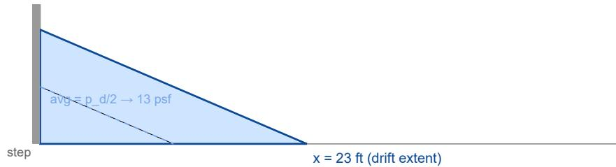
Triangular surcharge  $p_d \rightarrow 0$  over 23 ft. Total at step = 29.9 psf. For quick checks, uniform  $w = \frac{1}{2}p_d s = 91 \text{ plf}$  over 23 ft is acceptable.
