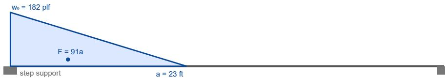
Model LC-S3 as triangular 0–23' from the step. For quick envelopes at the step support, it's acceptable to add  $F = 91a$  (lb) directly to the step-side reaction.
